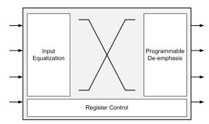
Fig. 2 - M21131/51 Device Architecture
