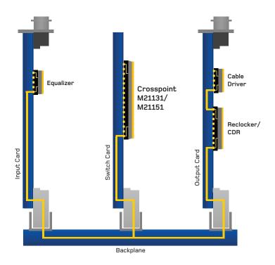
Fig. 3 - Routing Switcher Application Diagram
