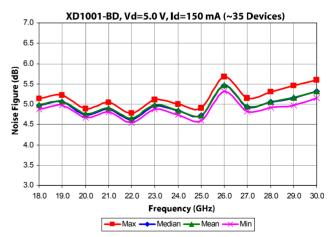
Note [1] Measurements – On-Wafer data has been taken using bias conditions as shown. Measurements are referenced 150 um in from RF In/Out pad edge. For optimum performance M/A-COM Tech T-pad transition is recommended. For additional information see the M/A-COM Tech "T-Pad Transition" application note.
