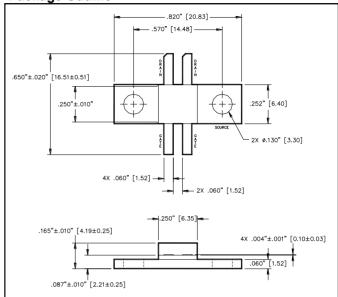
UNLESS OTHERWISE NOTED, TOLERANCES ARE INCHES ±.005" [MILLIMETERS ±0.13mm]
