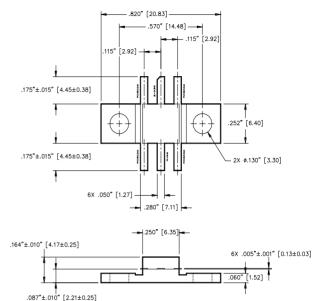
UNLESS OTHERWISE NOTED, TOLERANCES ARE INCHES  $\pm .005$ " [MILLIMETERS  $\pm 0.13$ MM]
