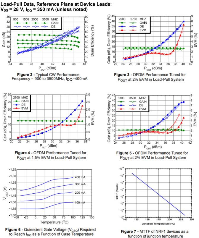
Load-Pull Data, Reference Plane at Device Leads:
