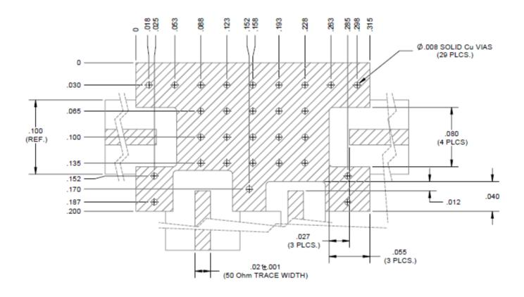
The hatched metal area on circuit side of device must be connected via lowest possible impedance to RF and DC ground. It also must be connected via lowest possible thermal impedance to the ambient temperature. Vias should be solid copper fill and gold plated for optimum heat transfer from backside of limiter module through circuit vias to heat sink on back side of PCB.
