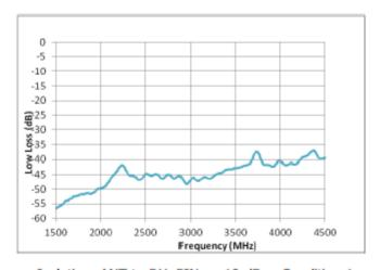
Isolation, ANT-to-RX, PIN = -10 dBm, Condition 1
