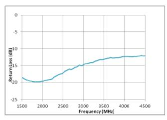
Return Loss, ANT-to-RX, PIN = -10 dBm, Condition 2
