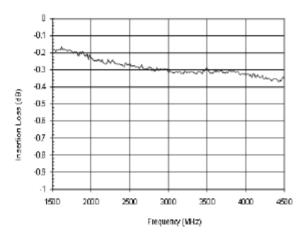
Insertion Loss, TX-to-ANT, PIN = -10 dBm, Condition 1
