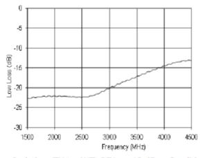
Isolation, TX-to-ANT, PIN = -10 dBm, Condition 2
