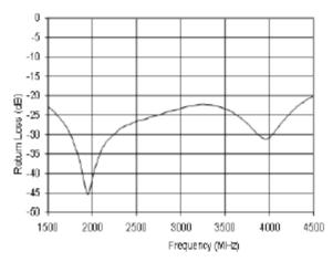
Return Loss, TX-to-ANT, PIN = -10 dBm, Condition 1
