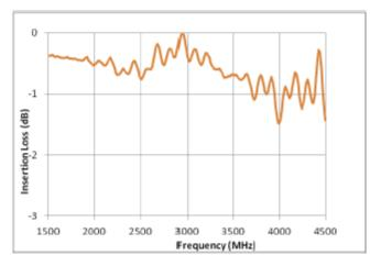
Insertion Loss, ANT-to-RX, PIN = -10 dBm, Condition 2
