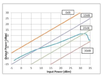
Output Power vs. Input Power, ANT to RX, Condition 2, f = 3.1 GHz
