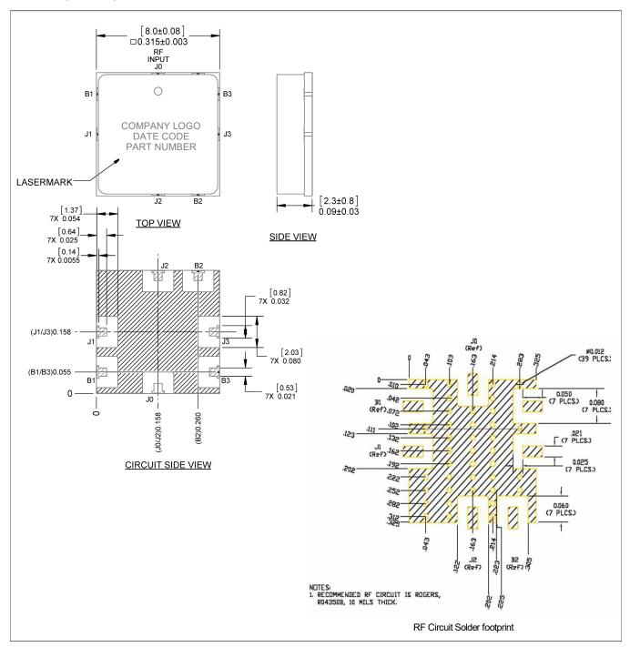
8. Hatched metal area on circuit side of device is RF, DC and thermal grounded.
