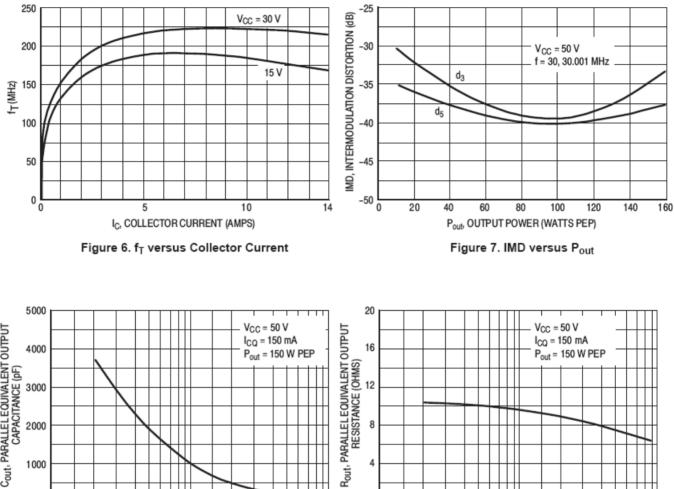
Cout, PARALLEL EQUIVALENT OUTPUT CAPACITANCE (pF) f, FREQUENCY (MHz) f, FREQUENCY (MHz)
