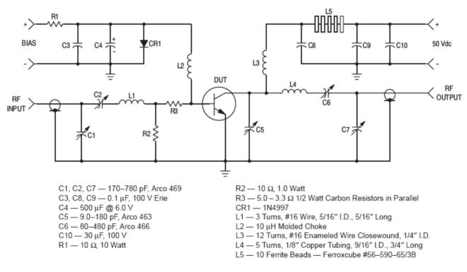
Figure 1. 30 MHz Test Circuit Schematic
