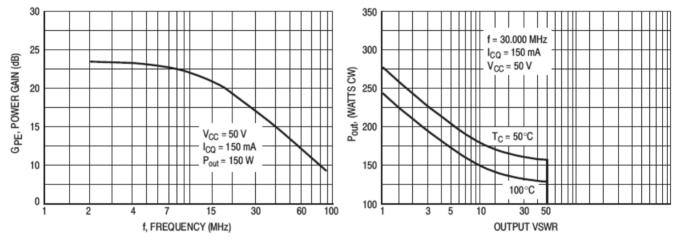
Figure 4. Power Gain versus Frequency
