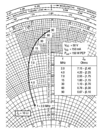
Figure 10. Series Equivalent Impedance
