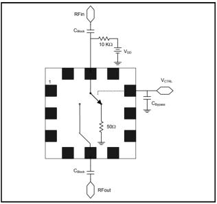
2. VDD can be injected at either pin 5 or pin 11.
