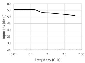
13.Input IP3 were measured using connectorized evaluation board with impedance matching. The RF input power was 14 dBm per tone with spacing of 1 MHz.
