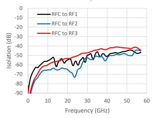
RFC to RF1 / RF3 / RF4 Isolation, RFC to RF2 On<sup>11</sup>
