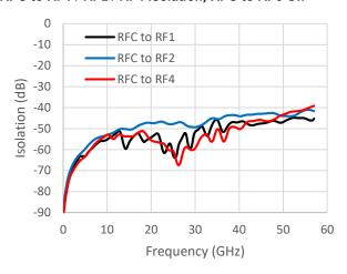
Isolation between RF1 to RF4, RFC to RF1 On<sup>11</sup>
