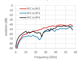
RFC to RF1 / RF2 / RF3 Isolation, RFC to RF4 On<sup>11</sup>
