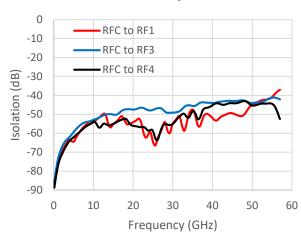
RFC to RF1 / RF2 / RF4 Isolation, RFC to RF3 On<sup>11</sup>
