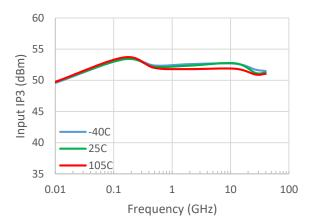
13.Input IP3 were measured using connectorized evaluation board with impedance matching. The RF input power was 14 dBm per tone with spacing of 1 MHz. The IP3 rolloff below 150 MHz is due to rolloff of test system IP3.
