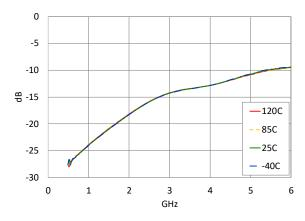
ANT to RX Insertion Loss over Current @ 25 °C, PCB Loss De-embedded
