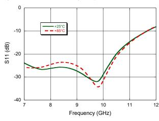
Output Return Loss vs. Frequency (Termination)
