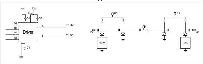
11. Recommended bias with this driver is  $V_{CC} = 5 \text{ V}$  and  $V_{EEB} = -30 \text{ V}$ .
