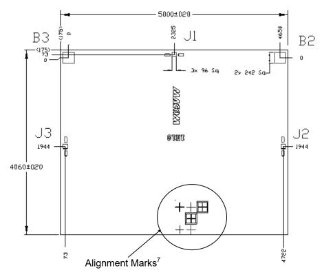
All dimensions shown in microns ( $\mu$ m). Thickness is 125  $\pm$  10  $\mu$ m.
