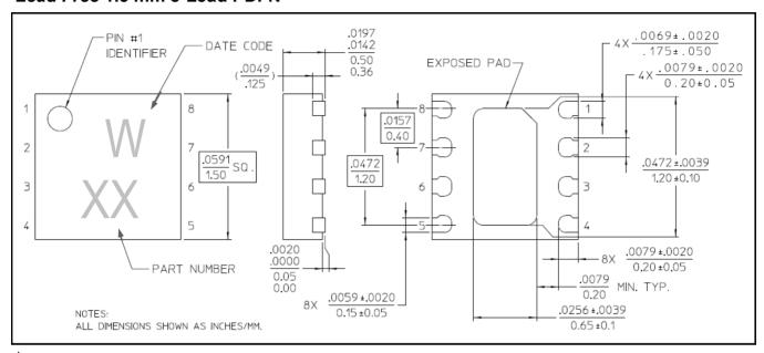
Reference Application Note S2083 for lead-free solder reflow recommendations and PCB footprint information. Meets JEDEC moisture sensitivity level 1 requirements. Plating is NiPdAu over copper.
