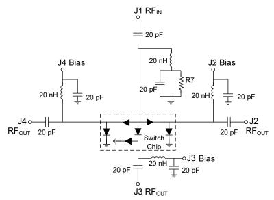
7. RLC values are for an operation frequency of 2 - 18 GHz and bias current of  $\pm$ 20 mA per port.
