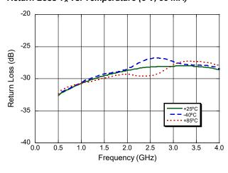
Return Loss R<sub>X</sub> vs. Temperature (5 V, 35 mA)
