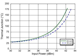
Input Power vs. PCB/Heatsink Temperature  $T_X = 5 \text{ V} @ 20\text{mA} & 30 \text{ mA}, R_X = 25 \text{ V} @ 0 \text{ mA},$  $T_X$  to Antenna,  $F_0 = 2010 \text{ MHz}$
