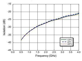
Isolation R<sub>X</sub> vs. Temperature (28 V, 0 mA)
