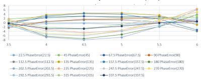
Following many traces, trying to consider how that will impact a system is difficult. A simpler method is adopted: RMS Error. It is important to use the right convention when applying an RMS calculation to phase shifter insertion phase. We compare the raw errors with the mean (error) below.
