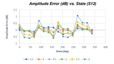
While the above shows amplitude error at particular frequencies vs phase shifter state, another common way to look at this parameter is error vs frequency.
