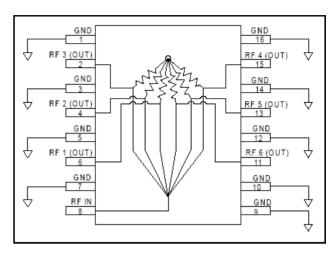
Pins 1, 3, 5, 7, 9, 10, 12, 14 and 16 must be DC and RF grounded.
