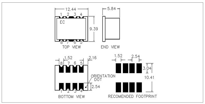
Dimensions in inches [mm]. Tolerance where not specified: .xx  $\pm$  .02, .xxx  $\pm$  .010
