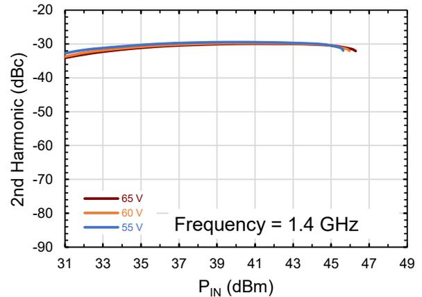
**Typical Performance Curves as Measured in the 0.96 - 1.4 GHz Evaluation Test Fixture:**
