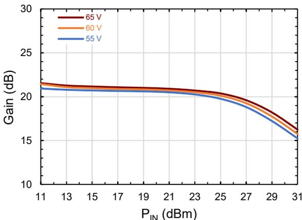
**Typical Performance Curves as Measured in the 0.96 - 1.4 GHz Evaluation Test Fixture**
