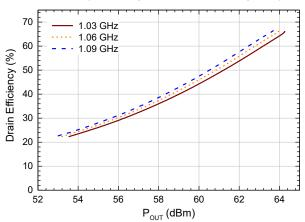
Drain Efficiency vs. Output Power and V<sub>DS</sub>
