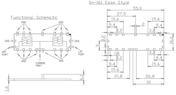
Dimensions in mm. Tolerance:  $.x \pm 0.1, .xx \pm 0.05$  Maximum coplanarity specification of 0.1mm
