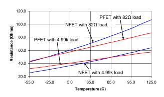
6. Output resistance were measured under the condition of  $V_{CC}$  = +5 V,  $V_{OPT}$  = +5 V, and  $V_{EE}$  = -5 V, with load resistors from outputs to ground.
