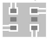
Recommended PCB layout shown above uses 1.6 mm FR4, Grounded coplanar wave guide, transmission line width 0.70 mm and gap 0.57 mm.
