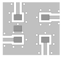
Recommended PCB layout shown above uses 1.6 mm FR4, Grounded coplanar wave guide, transmission line width 0.70 mm and gap 0.57 mm.
