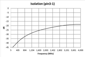
Electrical Specifications:  $P_{in} = 0 dBm$ ,  $T_A = 25$ °C,  $Z_0 = 75 \Omega$
