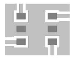
7. Recommended PCB layout shown above uses 1.6 mm FR4, rounded coplanar wave guide, transmission line width 0.70 mm and gap 0.57 mm.
