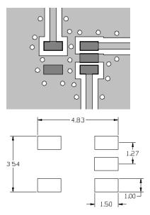
Recommended PCB layout shown above uses 1.6 mm FR4, Grounded coplanar wave guide, transmission line width 0.70 mm and gap 0.57 mm.
