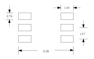
Recommended PCB layout shown above uses 1.6 mm FR4, Grounded coplanar wave guide, transmission line width 0.70 mm and gap 0.57 mm.
