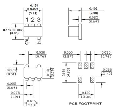
Dimensions are inches (millimeters)  $\pm 0.015$  (0.38) unless otherwise specified. Drawing not to scale.
