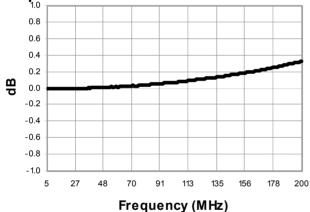
Insertion Loss 2: (Pin 1 to 4) 0.0 -0.1 -0.2 -0.3 -0.4 dВ -0.5 -0.6 -0.7 -0.8 -0.9 -10 91 113 5 27 48 70 135 156 178 200 Frequency (MHz)
