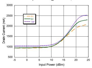
Drain Current vs. Input Power @ T = +25°C,  $V_D = 9 V$
