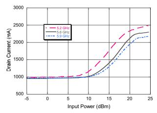
Drain Current vs. Input Power @ F = 5.6 GHz,  $V_D = 9$  V
