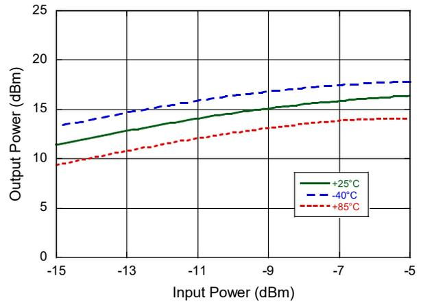
**Output Power vs. Input Power @ 42 GHz**
