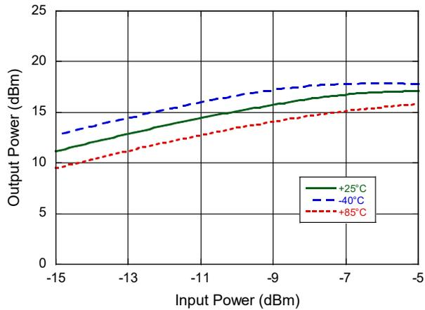
**Output Power vs. Input Power @ 35 GHz**
