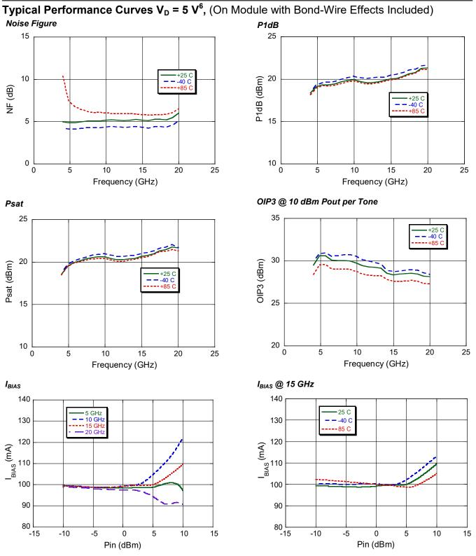
6. All plotted data is taken with the chip connected via two 0.025 mm (1 mil) wire bonds of minimal length 0.31 mm (12 mils) on the RF<sub>IN</sub> and RF<sub>OUT</sub> ports.
