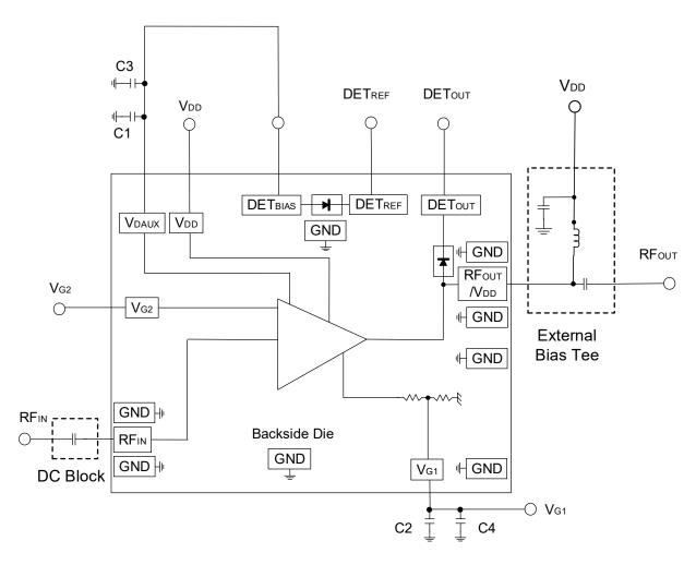
All bond pads labelled GND have vias to the backside metal. Bond wires on these pads are optional.
