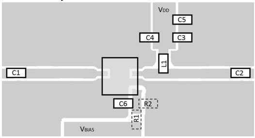
FR4, RF Layer Thickness = 0.711 mm, Trace = 0.55 mm, Gap = 0.18 mm
