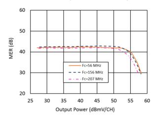
Pout @ 30 dB Modulation Error Ratio
