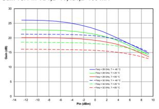
Pout vs. Pin VD1,2=4V, Id1,2=100 mA
