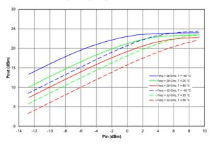
Gain vs. Pout VD1,2=4V, Id1,2=100 mA
