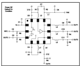
9. The exposed pad centered on the package bottom must be connected to ground for RF, DC and thermal considerations.
