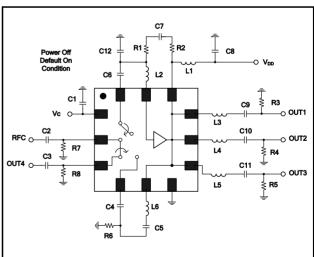
10. The exposed pad centered on the package bottom must be connected to ground for RF, DC and thermal considerations.
