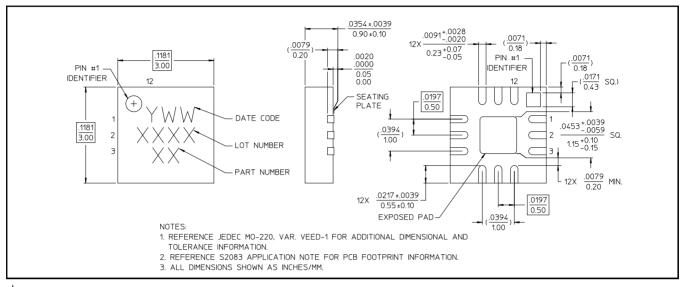
Reference Application Note S2083 for lead-free solder reflow recommendations. Meets JEDEC moisture sensitivity level 1 requirements. Plating is 100% matte tin over copper.
