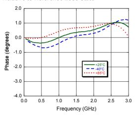
Phase - 31 dB Attenuation vs. Frequency Relative to Reference Loss State
