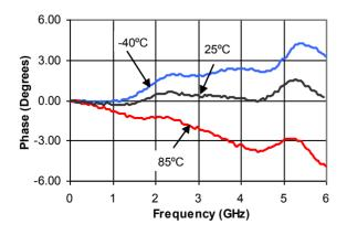
Phase - 1 dB Bit vs. Frequency Relative to Reference Loss State
