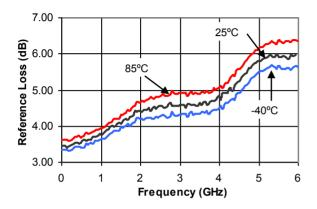
Attenuation - 2 dB Bit vs. Frequency
