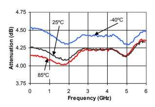
Attenuation - 16 dB Bit vs. Frequency
