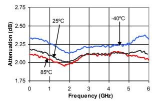
Attenuation - 8 dB Bit vs. Frequency
