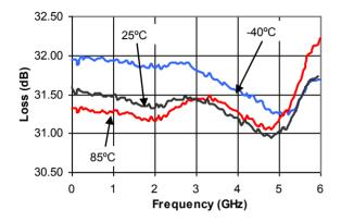
Phase - 2 dB Bit vs. Frequency Relative to Reference Loss State
