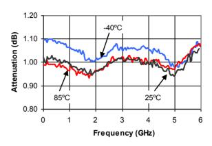
Attenuation - 4 dB Bit vs. Frequency
