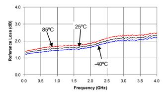
Attenuation - 2 dB Bit vs. Frequency
