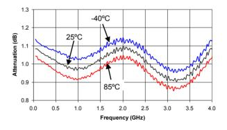
Attenuation - 4 dB Bit vs. Frequency
