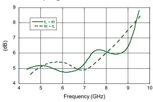
Conversion Loss vs. Frequency (Up Conversion) IF = 1 GHz, Input to I-Port, LO Power = 20 dBm
