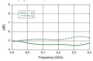
Conversion Loss vs. Frequency (Down Conversion) IF = 2 GHz, Output @ I-Port, LO Power = 20 dBm
