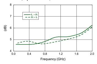
Conversion Loss vs. Frequency (Down Conversion) IF = 1 GHz, Output @ I-Port, LO Power = 20 dBm
