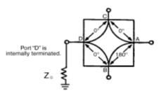
Figure 1. 2-way, In-Phase (180°) Power Divider/Summer, or ISO-T
