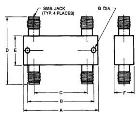
All dimensions are ± .020 except mounting diameters (± .005) and mounting hole location (± .010).
