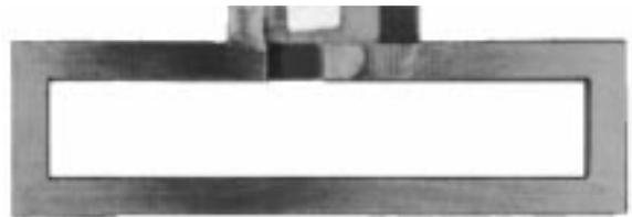
Line Transformer on P.C. Board (Figure 29)
