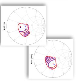
(Above) Load pull Pout and PAE using MACOM MAPC-A1101 packaged transistor device
