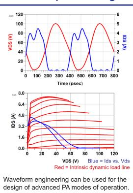
Intrinsic voltage and current access allows for simulation of the waveforms and dynamic load line.
